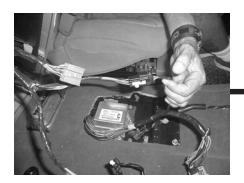
**STEP I1:** As the console is tilted up, there are more wiring harness that are exposed and that need to be disconnected.
